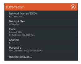
To view and change internal wireless detail values (Network name (SSID), Network key, or Channel) the internal wireless must be in **Access Point** (Internal Wifi) mode. To select a network (hotspot) to connect to, the internal wireless must be in **Client Mode**.
