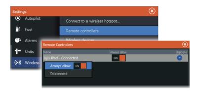
Selecting **Always allow** means the device can automatically connect without needing a password each time. This menu also allows disconnection of devices that no longer require access.
