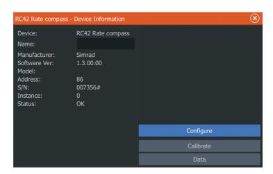
All devices allow allocation of an instance number in the **Configure** option. Set unique instance numbers on any identical devices on the network to allow for the unit to distinguish between them. The **Data** option shows all data being output by the device. Some devices will show additional options specific to the device.
