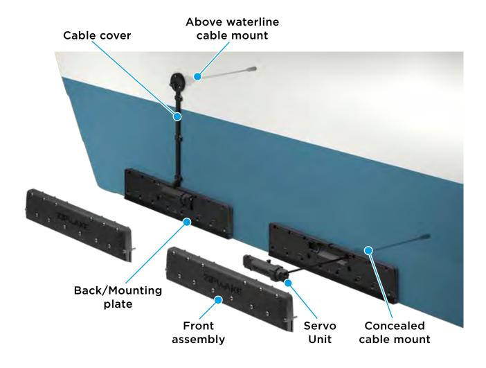
For best effect, different size interceptors can be combined to span as much of the transom edge as possible. A full beam is always the optimal arrangement from a lift-to-drag ratio point of view.
